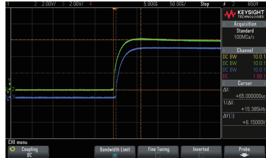
▲ channel synchronization plus rise time as fast as 65µs
